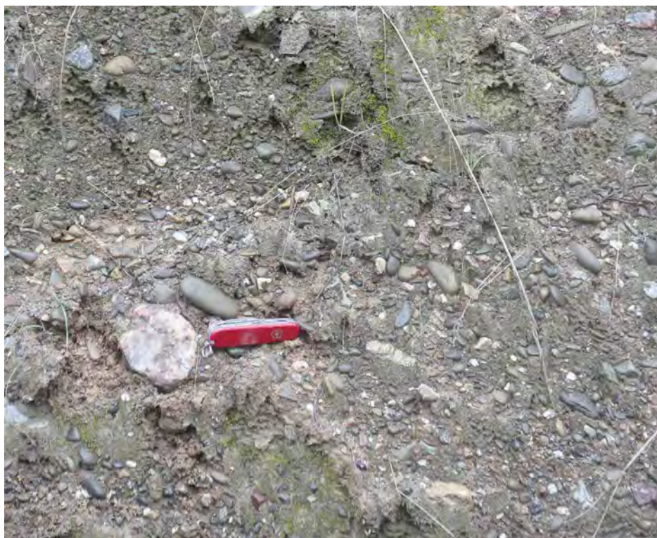
Photo No. 4 Sandy clayey gravel near northwest end of proposed Arroyo del Valle realignment (January 2017)
