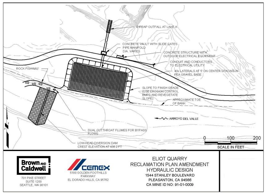
SOURCE: B&C 2020, Hydraulic Design Study Figure E-2; modified by Benchmark Resources in 2020. NOTE: Figure is not printed to scale.
